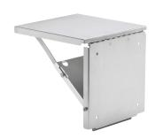
Stainless Steel Folding Shelf is an ideal accessory to support laptop computers, monitoring units and other equipment used to install and maintain electrical components in an enclosure. The shelf can be installed on the inside or outside surface of Free-stand or Floor-Mount enclosures (except ProLine). It automatically locks in the horizontal position when raised. When not in use, the shelf takes up minimal space and folds to 1.00 in. (25 mm) from the mounting surface.
