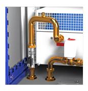
The stainless steel pipe inserts with ID 1" each come with a pair of ratiometric liquid coolant sensors. The sensors connect directly to the RackChiller Rear Door Controller. This enables monitoring of the coolant thermal properties and cooling. performance, as well as additional temperature control features.
