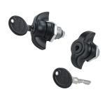
The Keylocking Quarter-Turn Wing Knob locks a variety of wall-mounted enclosures. The Wing Knob includes a gasket, mounting nut and one key with the 333 key code. This Wing Knob should be used with an existing cam for installation; please note the cam is not included with Wing Knob. It can be locked in the open or closed position. This product maintains the cabinet rating Type 4, 12.
