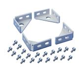
The ProLine Frame Floor-Mounting Bracket provides a structural method of bolting a ProLine frame to the floor. The bracket fits all frame sizes, the kit includes four brackets and mounting hardware. This bracket is not to be used with colocation frames, which include welded-in floor mounting brackets.
