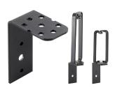
The Universal D-Ring Bracket mounts D-Ring's (order separately) on ProLine or Network Vertical Tie-Down Cable Manager, ProLine Front-to-Back D-Ring Bracket or grid strap. The D-Ring locks into hole provided on the bracket, creating support for cable management. It is made of steel, coated with RAL 9005 black polyester powder paint and includes mounting hardware.
