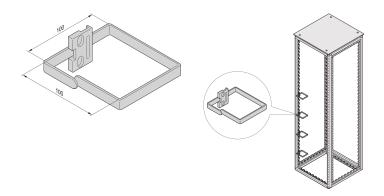
Cable eyes for free standing racks to support vertical structured cable management along the Varistar frame uprights.
