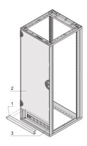
Door Hinge Bracket for shortened Doors, Heavy-Duty and Slim-Line, Front or Rear.
