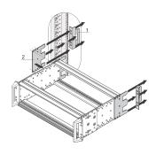
Adapter for rear fixing of a subrack in accordance with DL3 standard into a cabinet. It guarantees shock and vibration resitance up to 25 g.
