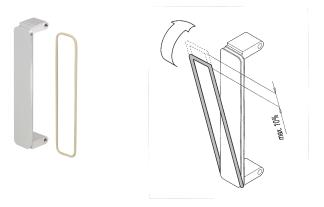
The O-ring gasket can be used for EMC shielding of PMC or FMC mezzanines. The O-ring will be assembled into the groove of the Mezzanine.
