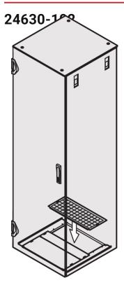
Filter Mat helps cover the openings in the base plate which is otherwise used for cable management.
