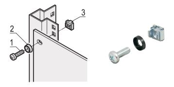
For standard grounding use a grounding nut and washer on at least one attachment point.
