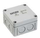
nVent RAYCHEM JB16-02 and JB-82 temperature-resistant polycarbonate junction boxes for non-hazardous areas. For use with nVent RAYCHEM self-regulating heating cables, to make a power connection, tee, splice, powered splice/tee. Up to four heating cables, or three heating cables and the appropriate size power cable can be connected through the four entries and connected to the rail mounted terminals.
