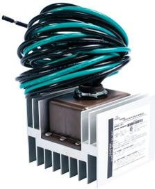
RAYCHEM 920 Series - SSR provides electronic switching capability for heat trace circuits. Available in 1-,2-, or 3-pole solid-state, normally open relay , 277V or 600V, and 30A or 60A at 104°F (40°C). Allows for proportional, power limiting, and soft start control algorithms.
