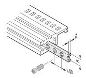
The threaded insert is a metal strip with thread M3 and allows the fixing of front panels.
