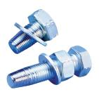
The ELFB taper bolt is used to firmly attach a nVent LENTON taper-threaded coupler onto formwork in precast and cast-in-place construction. This reusable form saving accessory allows forms to be pre-drilled with the correct spacing of the reinforcing steel, which speeds construction and allows the forms to be re-used on repetitive construction elements. This system can be used in conjunction with coupler boxes to eliminate the use of bend-out-boxes and also helps eliminate protruding dowel bars.
