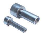
The nVent LENTON D16A Mechanical Anchor with Extension provides a method of splicing and anchoring reinforcing bar in segmental concrete construction applications that have limited space or are severely congested. The large head significantly reduces required embedment lengths. The anchors are a combination of standard nVent LENTON Terminator D16 Mechanical Anchors and ELFM Female-to-Male Extensions.
