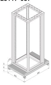
Aluminum mobile base plinth with load capacity of 300 kg, for aluminum cabinets with 600 mm breadth.
