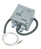
nVent RAYCHEM T-M-10-S/+x+y is a non-hazardous area mechanical surface sensing thermostat providing temperature control for heating cables. Available in ranges: 0 °C-50 °C; 0 °C-200 °C; 50 °C-300 °C. The temperature set point can be adjusted without opening the enclosure via a removable plug in the lid. Direct connection of the heating cable is possible, switching current capacity is 16 A.
