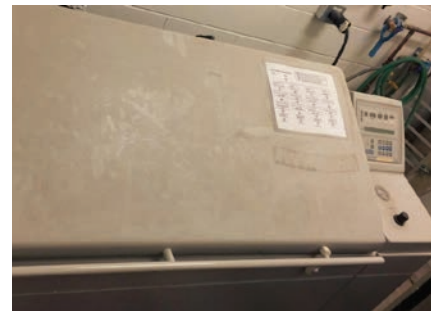
Figure10: Salt Fog Corrosion Chamber[5]
