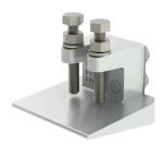
The nVent ERICO Telecom Flange Clamp is designed to provide a grounding connection point to: 1) curved flanges that may exist on steel monopole telecommunication towers and 2) straight flanges that exist on towers constructed from angled steel. The clamp is an integral part of the tower grounding system used to ground & bond antennas, nVent ERICO Tower Mounted Ground Bars, and telecommunication equipment to the tower.
