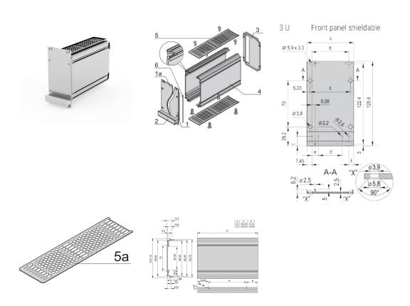
Protects a PCB against mechanical damage and discharges electrostatic buildup; for Euroboard formats; pair panel with one cutout for one connector.
