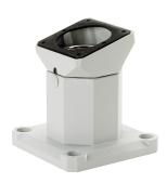
Compact Series 2 Rotational Base Bracket, 15-degree attaches the enclosure directly to a horizontal surface, enabling 300-degree enclosure rotation and 15-degree angle tilt
