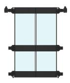
Designed for 48-inch (1200mm) wide aisles. Can also provide benefits for wider aisles. A 48-inch (1219 mm) wide version seals aisles from 46-inch (1168 mm) to 54-inch (1372 mm) and a 72-inch (1829 mm) wide version seals aisles from 70-inch (1778 mm) to 78-inch (1981 mm). Custom solutions can also provide benefits for wider aisles.
