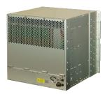
Rugged VPX system for 10 VPX boards 6 U, 1", 160 mm and 10 Rear I/O boards. The power for the system is supplied by a pluggable VPX power supply. A fan control module monitors the fans, the temperature and voltage.
