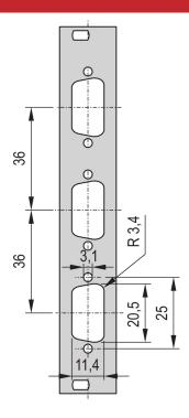
19" Front Panel with SUB-D Cut-Out or FDDI Cut-Out.
