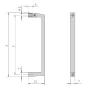
Slim Aluminium profile front handle, 7 mm. The assembly of the handle will be done from the rear side.
