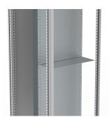
This steel zink plated separation plate, MSISM, is available off the shelf and pre-sized. The plate should be used when subsections need to be segregated. It is placed between a mounting plate and a front panel that is placed inside the enclosure. No screws are needed, which makes mounting easy. The fix section can then comply to up to form 4 segregation according to IEC 61439.
