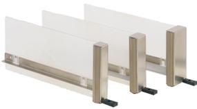
This AdvancedMC filler module consists of a stainless steel front panel without LEDs and has EMC gaskets on the left hand and bottom side. The filler module is fixed into the chassis card guide by a snap in plastic nose. The module can be used to cover an empty slot, to ensure EMC shielding and close the front to seal air leaks into the chassis. These filler modules can be used in AdvancedMC Carriers and in MicroTCA slots. It doesn't require a locking bar.
