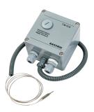
nVent RAYCHEM T-M-10-S/+x+y is a non-hazardous area mechanical surface sensing thermostat providing temperature control for heating cables. Available in ranges: 0 °C-50 °C; 0 °C-200 °C; 50 °C-300 °C. The temperature set point can be adjusted without opening the enclosure via a removable plug in the lid. Direct connection of the heating cable is possible, switching current capacity is 16 A.
