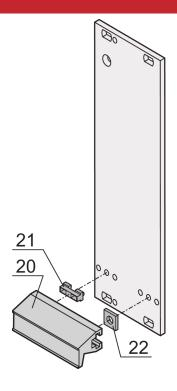
The static Alu-profile handle, trapezoid form can be mounted to a front panel for extraction of the PCB.
