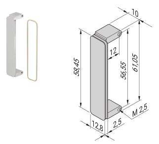
A FMC bezel is fitted into FMC mezzanine front panel cutouts, Kit of 10 FMC bezels.
