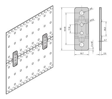
The brackets are used to connect the fan units to the side panels of a subrack.
