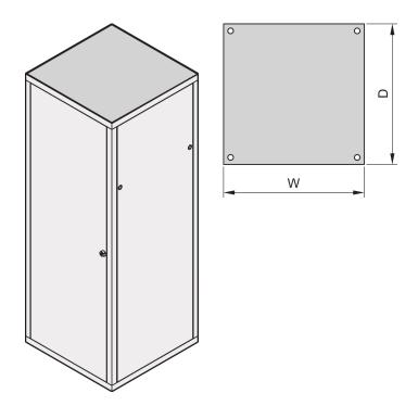
Flush top covers are used for enclosures with less electronic density where cooling is not a necessity. Additionally as the cover is laid into the frame, it consumes less spave vertically and is more asthetic.
