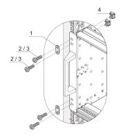
For fixing a subrack with dual fixing holes to 19" mounting brackets (e.g. rugged and railway subracks).
