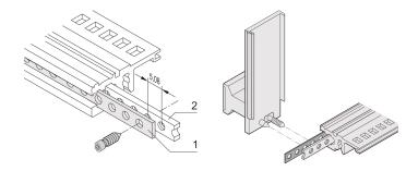
Perforated strip out of 1mm Aluminum for centering shielded plug-in units.
