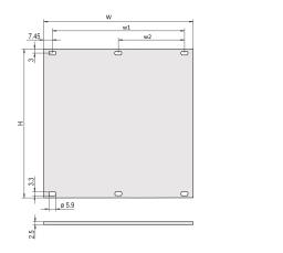
Front panel, unshielded, front anodized and rear conductive.
