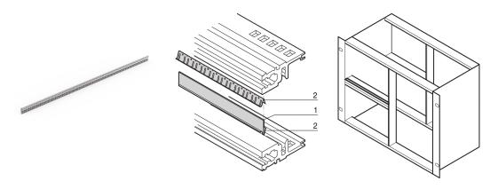
The contact strip makes contact bewteen horizontal rails. If two horizontal rails are mounted one above the other, the seals plus a metal strip enable EMC shielding.
