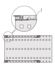
Mechanical covering of installed components. The plate is inserted into a groove of the L type horizontal rails.
