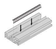
Stainless steel gasket is clipped into a groove of horizontal rail and enables contact to the cover plate.
