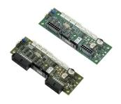
Management Module for Fan Control and Voltage Monitoring.
