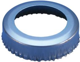
Packing caps are used when splicing to short dowels and there is not enough room for standard installation equipment. Packing caps help retain and position packing materials, which helps minimize leakage of the molten filler materials during installation.
