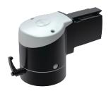
Syspend 281-Max Flange Elbow Coupling attaches directly to the enclosure for applications where a vertical tube is not required. Enables enclosure to be rotated 300 degrees and locked in position. Includes safety stop and maintenance-free bearing.
