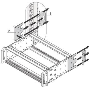
Adapter for rear fixing of a subrack in accordance with DL3 standard into a cabinet. It guarantees shock and vibration resistance up to 25 g.
