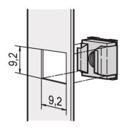
Cage nuts permit range of choice of nut and bolts sizes and easily replaced unlike pre-threaded holes. Cage nuts are easy to use on materials too thin or soft to be threaded.
