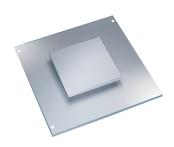
Pagoda tops can be used on the top of a modular enclosure for active cooling. The design features a drip-proof raised pagoda vent with a 115-volt integral axial exhaust fan, and includes gasket seals to maintain a NEMA 12 enclosure rating.
