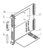
Voltage keying/coding pin for PMC mezzanine boards.
