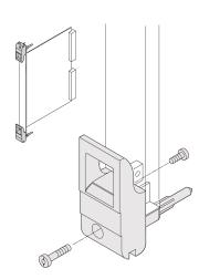
The inserter/extractor handle, type IET in accordance with IEEE 1101.10. 0,1" offset. Two of these handles can overcome a single lever force of 700 N (per pair).
