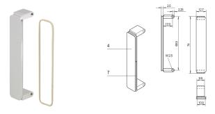
Mezzanine front panel is fitted into PMC front panel cut-outs. Available in different treatments.
