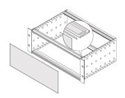
The contact strip clips onto the horizontal rail and makes the contact to front or rear panel.
