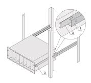
The C-profile, assembled on the Side Panel of the subrack serves fixes the subrack on the guiding profile when mounted into a cabinet.
